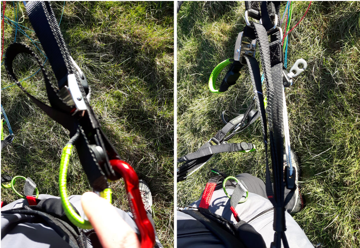
Niviuk ROLLER trimmers: standard cam buckle with a magnetic tail to prevent flapping strap [updated risers, Dec 2016].
